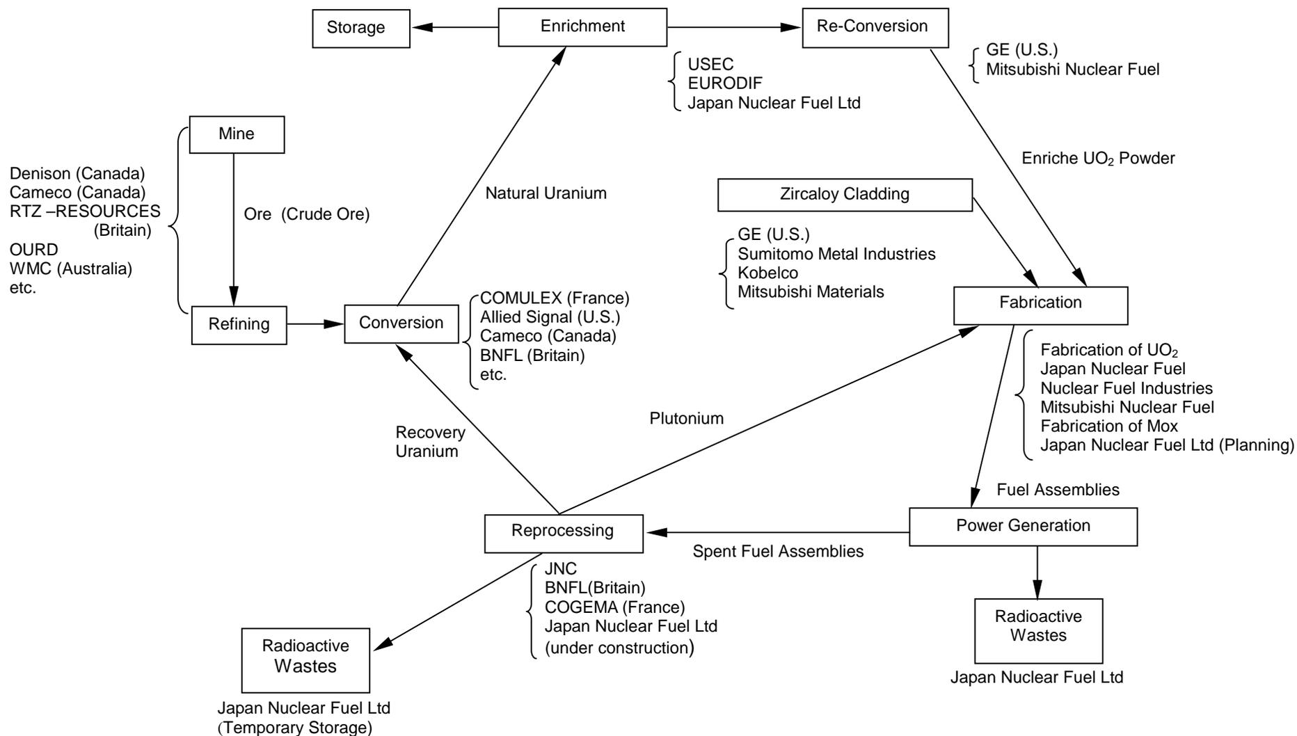
FIG. 6. Nuclear Fuel Cycle Diagram
